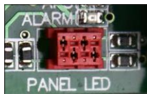
Gniazdo panelu LED
